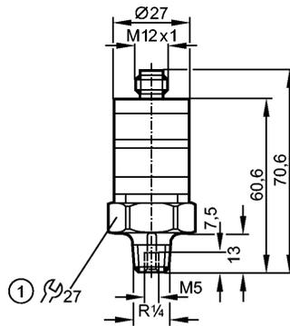
1: tightening torque 25 Nm
