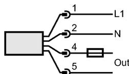
Note: miniature fuse to IEC60127-2 sheet 1, ≤ 5 A (fast acting)
