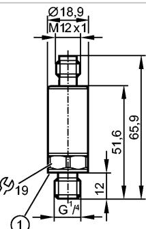
1: Process connection sealing FKM / DIN 3869
