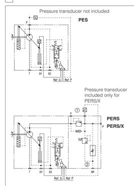
Digital P/Q controller integrates the alternate pressure and flow regulation with the electronic max power limitation.
