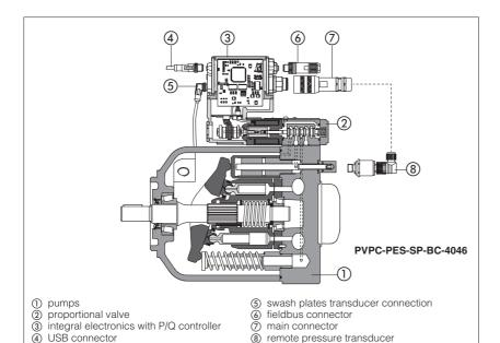
The variable displacement axial piston pumps type PVPC, can be supplied with advanced electrohydraulic proportional controls:
