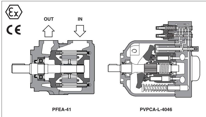
PFEA vane and PVPCA piston pumps are certified for application in potentially explosive atmospheres according to ATEX 94/9/CE, protection mode Ex II 2/2 GD cbk IIC T6/T5/T4 (group II for surface plants with gas, vapours and dust environment, category 2, zone 1, 2, 21 and 22).
