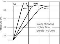
Above indications have to be considered as a general guideline, being affected by hydraulic circuit stiffness, working flow and dead volume. The valve's dynamics can be further optimized on the specific application, customizing PIDs parameters.
