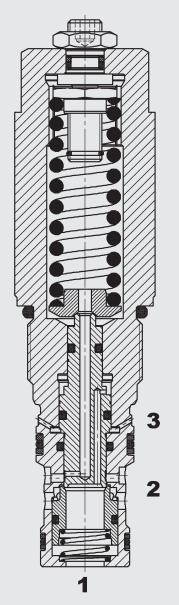
The counterbalance valve RSM12121 is a direct-acting poppet valve. Its function is to control the speed of a consumer according to the inlet flow. It also prevents the consumer from overrunning if there are pulling loads and ensures smooth action in consumers. In addition it fulfils the function of a hose-break valve.
