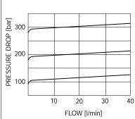
The Performance Chart illustrates flow handling capacity at max. setting for each spring range option. Pressure rise will vary with spring (range) and with setting within range due to flow forces.
