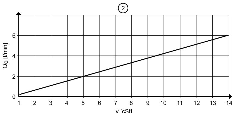
Response threshold  $Q_{\min}$  depending on the kinematic viscosity
