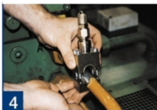
4 clamp SC onto pipe
