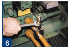
6 screw the valve to the right until it stops then screw it to the left
