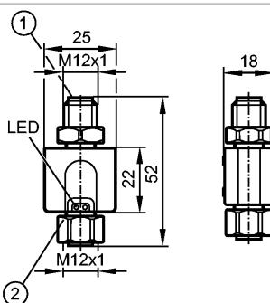
1: connection for voltage supply and output signals
