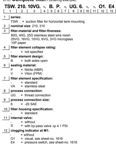
To add an indicator to your filter, use the corresponding indicator data sheet to find the indicator details and add them to the filter assembly model code.
