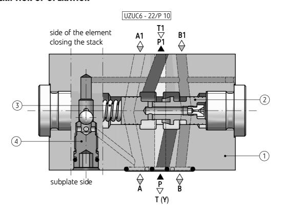
Main elements of the valve type **UZUC6**... are body (1), spool (2), spring (3) and logic valve (4) used to select higher control pressure from port **A** or **B**. For version UZUC6...**P**... (2-way version) the difference of pressures between port P and ports **A** or **B** acts on the spool (2), and after the initial spring (3) tension is overcome, the
