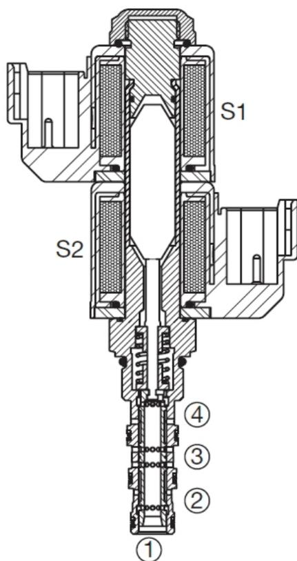
In de-energized mode the ports 2 and 4 are blocked – whereas there is flow from port 3 to 1 and in opposite direction.
