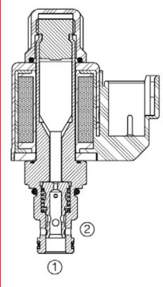
In de-energized mode the valve is blocked in both directions. If energized, the valve opens and allows the flow in both directions.
