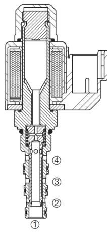
In de-energized mode, the valve allows flow from port 1 to 2 and from 3 to 4 and also in the opposite direction. If energized, the valve allows flow from port 1 to 4 and from 3 to 2 and also in the opposite direction.
