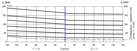
p = f(Q) Pressure - Flow rate characteristic [ $p_N = 250$  bar]
