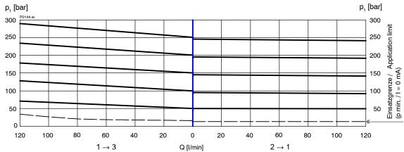
p = f(Q) Pressure - Flow rate characteristic [ $p_N = 350$  bar]
