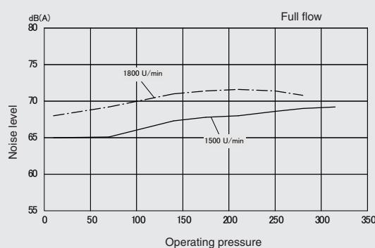
\* measured with noise level meter 1 metre away from pump in an anechoic room using a flexible coupling to DIN45635
