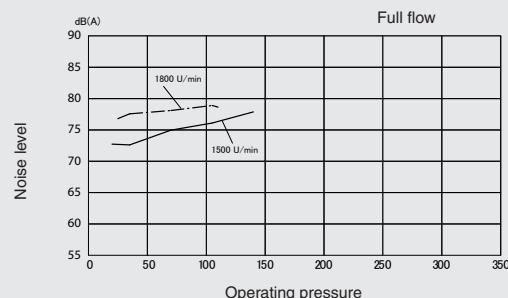
\* measured with noise level meter 1 metre away from pump in an anechoic room using a flexible coupling to DIN45635
