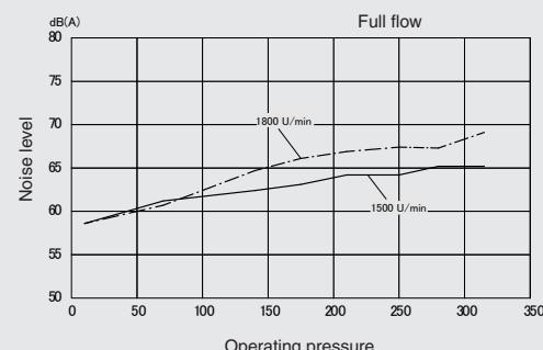
\* measured with noise level meter 1 metre away from pump in an anechoic room using a flexible coupling to DIN45635
