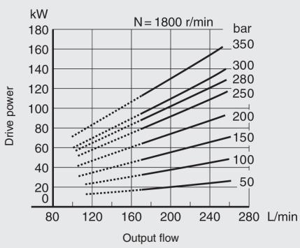
Note: The dotted lines in the graph are below the minimum adjustable flow
