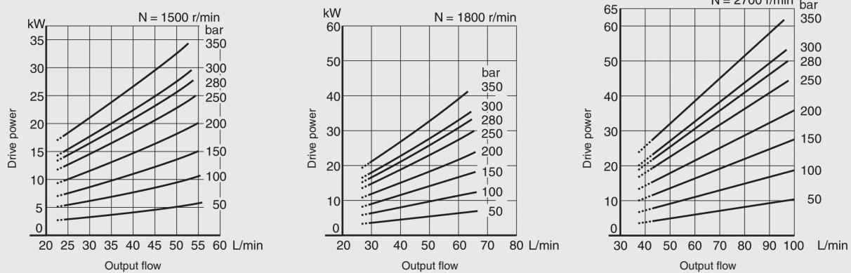
Note: The dotted lines in the graph are below the minimum adjustable flow
