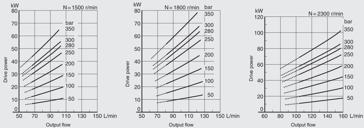
Note: The dotted lines in the graph are below the minimum adjustable flow
