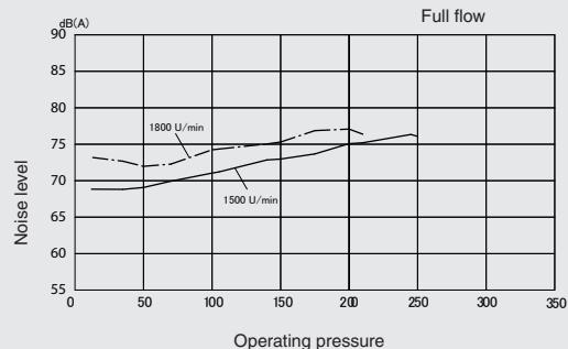
\* measured with noise level meter 1 metre away from pump in an anechoic room using a flexible coupling to DIN45635
