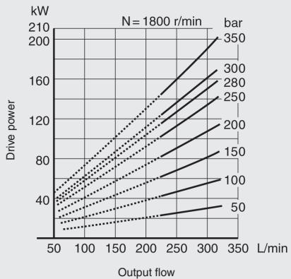
Note: The dotted lines in the graph are below the minimum adjustable flow
