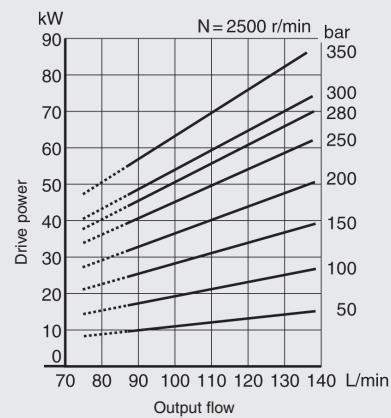
Note: The dotted lines in the graph are below the minimum adjustable flow
