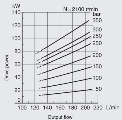
Note: The dotted lines in the graph are below the minimum adjustable flow
