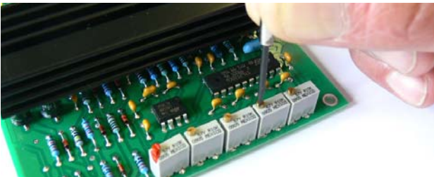
The trim potentiometers (P1) that are sealed with colour spots are preset in the factory.
