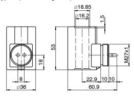
Coil with connection AMP Superseal / Metri Pack 150, 2-pole
