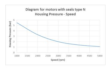
Different housing pressures and different drain fluid temperatures can be achieved with different Seals. With seals type N (Nitril seals) maximum drain fluid temperature is 75°C.
