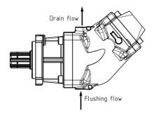
In order to provide an additional cooling flow to the rotating parts of the motor, when it operates at high speeds a housing flushing valve must be considered. Housing flushing can be achieved through a flushing valve or through a connection between the return line and the flushing plug.
