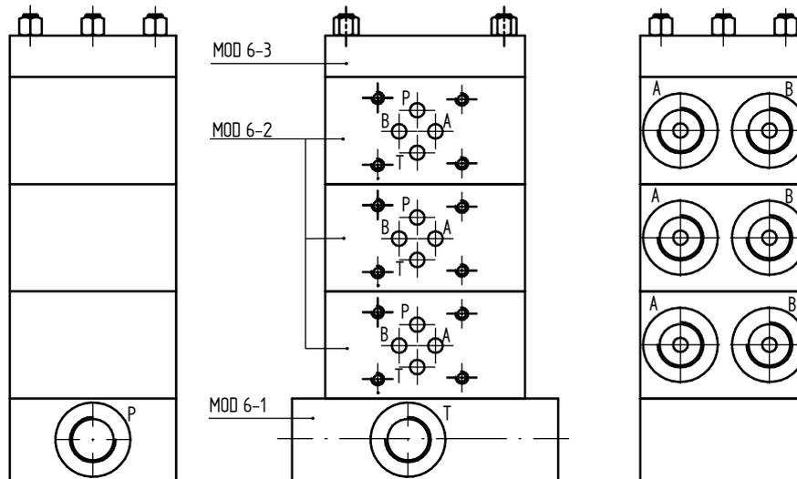
Below hydraulic equipment manufactured by PONAR Wadowice that can be used for control systems to be mounted on the multi-station manifold block:
