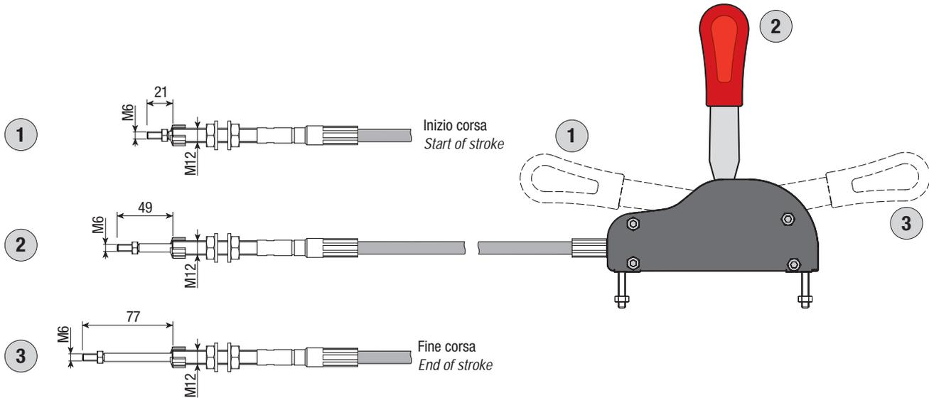
**CORSA TOTALE 56 mm / TOTAL STROKE 56 mm**
