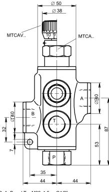
Size of ports P, A, B and T = M22x1,5 or G1/2" Weight: 2,6 kg
