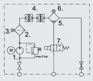
**INLET** Drain, water **OUTLET** G1/2" OIL G1" OIL G1"
