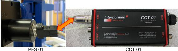
Connect the analogue outputs of the CCT 01 (CON 1 - interface) with your evaluation system. (see chapter 5.2)
