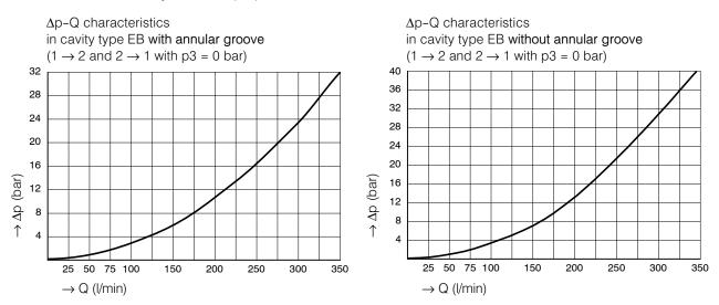
The  $\Delta p$  characteristic is valid when the load pressure in the connection  $1 \rightarrow 2/2 \rightarrow 1$  is greater than the opening pressure. If the load pressure is less than the opening pressure, the load pressure must first rise to overcome the opening pressure before flow can occur.
